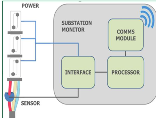
**Figure 2: Master Control Unit (MCU) for PQ data communication**
