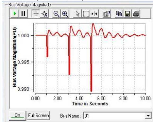
**Figure 1: Transient waveform analysis during PQ monitoring**
