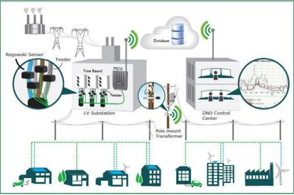
Figure 5: Schematic layout of PQ monitoring using transient analysis
