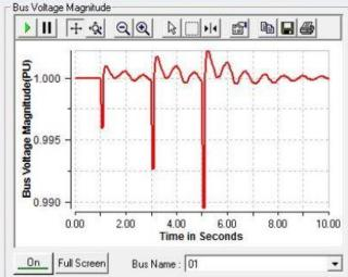
Figure 1: Transient waveform analysis during PQ monitoring
