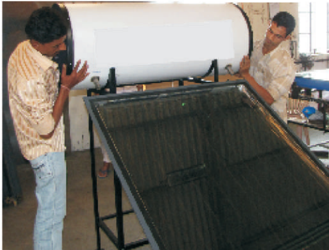
e. Assembly of the collector with stand and installation.
