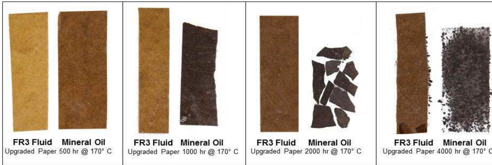
FR3™ natural ester fluid vs. Mineral oil Sealed Tube Test – ML 152-2000
